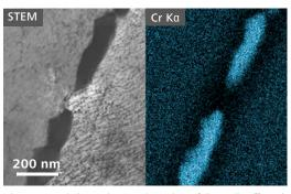
Chromium carbides at the grain boundary of thermally-affected X2CrNi18-10 steel: STEM BF in a FIB-SEM (left), EDS chromium map (right).
