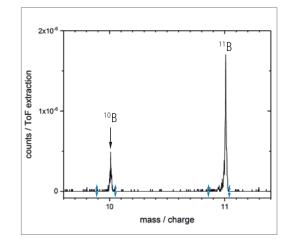
SIMS spectrum of boron doped silicon. The peaks at 10 and 11 amu correspond to the two isotopes of boron. The concentration of <sup>10</sup>B is below 4.2 ppm.
