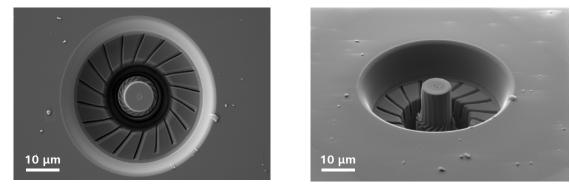
Pillar for compression testing after being machined using lathe milling: SEM top view (left), SEM side view (right).
