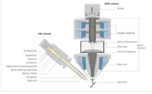
ZEISS Crossbeam 550: FIB- and FE-SEM column arranged at an inclination angle of 54°.
