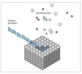
Working principle of SIMS: The Ga focused ion beam (blue) removes material from the top few nm of the sample surface. Different sputtered ion species (light and dark grey) are collected and transferred to the ToF-SIMS detector.
