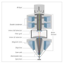
ZEISS Crossbeam 550: Gemini II column with double condenser and two Inlens detectors.
