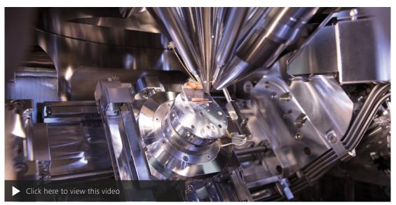
Find your region of interest quickly with the help of the super-eucentric 6-axis stage and always stay at eucentricity when tilting the sample. Prepare your sample. Lift out your TEM lamella, eventually.
