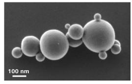
Alumina nanospheres imaged at 1 kV and FIB-SEM coincidence point with Tandem decel exemplifies high resolution, surface sensitive imaging of challenging samples.
