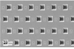
Array of TEM lamellae fabricated with automated preparation.
