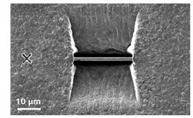
Lamella of a copper sample ready for lift out, fabricated with automatic sample preparation, prepared and imaged by FIB.
