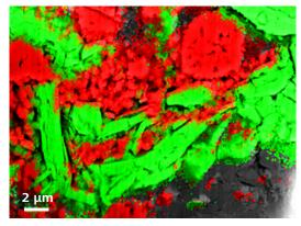
*LiMn*<sub>2</sub>O<sub>4</sub> cathode material of a lithium ion battery. Close-up of cross-section shows surface information on an Inlens SE image and unique, pure materials contrast with an Inlens EsB image. The distribution of lanthanum (red) and manganese (green) is derived from an EDS map (from left to right).
