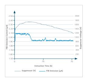
Regulation characteristic of Ga source emission current. The suppressor voltage regulates the total emission current between 1.9  $\mu$ A and 2.1  $\mu$ A.
