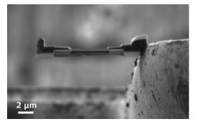
Ion-sculptor 5kV image of a lamella of poly-crystalline silicon. High imaging quality at low voltages allows precise thinning of the central region of the lamella.
