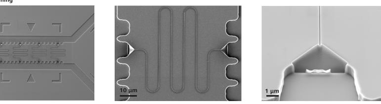
Nanofluidics channels fabricated by FIB in a silicon master stamp (left). Detail: meander-shaped channel (center). Inlets and outlets have a funnel shape (right). Courtesy of: I. Fernández-Cuesta, INF Hamburg, Germany.
