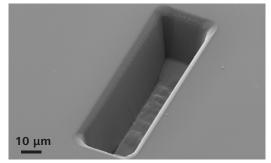
Trench milled in silicon, dimensions  $100 \times 30 \times 25 \ \mu m^3$ , milling time 10 minutes using 100 nA FIB current.
