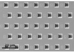
Array of TEM lamellae prepared automatically.
