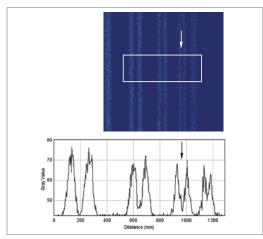
Top: Al (27 amu) map of a calibrated BAM L200 sample. The FOV is 2 μm. Bottom: Line profile for the area within the green frame. Lines with a width and separation of 33.75 nm can be resolved clearly (arrows).
