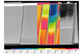
Use SmartEPD to determine the lamella thickness and endpoint of polishing quantitatively.
