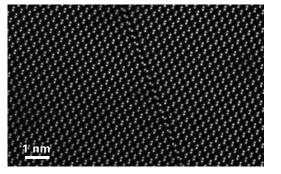
Silicon in <110> orientation, STEM image of a FIB lamella in a TEM. <110> silicon dumbbells and a twin boundary are clearly visible. The TEM lamella was prepared with the lon-sculptor FIB of ZEISS Crossbeam 550 with low kV thinning. Image Courtesy of: C. Downing, CRANN Institute, Trinity College, Dublin, Ireland. Nion UltraSTEM 200.
