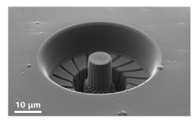
Pillar for compression testing after being machined using lathe milling.
