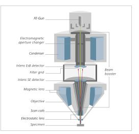
ZEISS Crossbeam 350: Gemini colum with single condenser, two Inlens detectors and VP capability.
