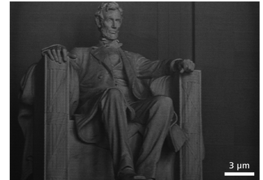
A FIB grayscale rendering of the Lincoln Memorial is patterned into silicon with the FIB beam. An unmodified photograph was used as the data source. Patterning time: 10 minutes.
