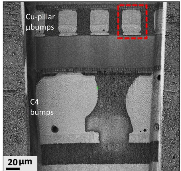
Figure 2b: Backscattered electron SEM image of package interconnect consisting of Cu-pillar microbumps and C4 bumps, immediately after laser processing and correlating to the area defined in Fig. 2a. Scale bar: 20  $\mu\text{m}$ .
