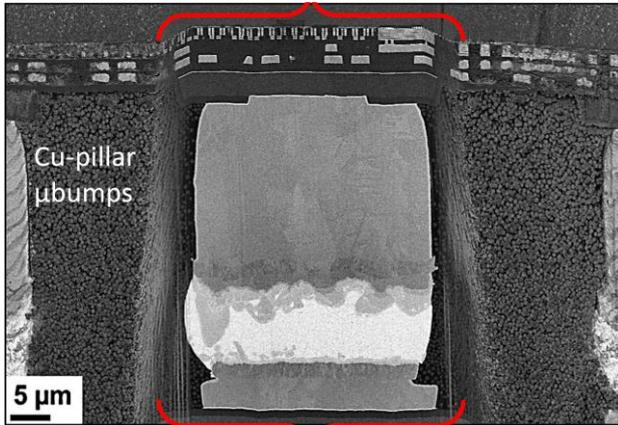
Figure 2c: Backscattered electron SEM image of Cu-pillar microbump (outlined in Fig. 2b) after Ga-FIB polish. Scale bar: 5  $\mu\text{m}$ .
