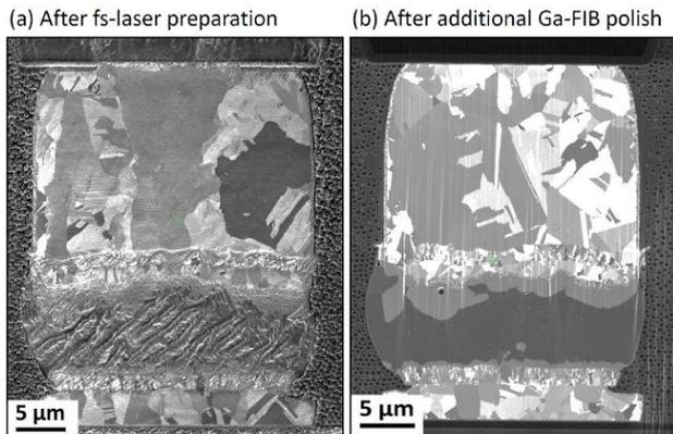
Figure 3: FIB secondary electron image series comparing the cross-section quality directly after fs- laser processing (a) and after an additional Ga-FIB polish step (b). Scale bars: 5  $\mu\text{m}$ .
