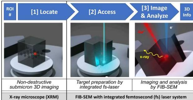
Figure 1: Schematics of the correlative workflow combining 3D XRM (step 1), femtosecond laser preparation (step 2), FIB polishing and SEM imaging and analysis (step 3).
