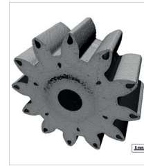
Entire sample (low resolution XRM)
