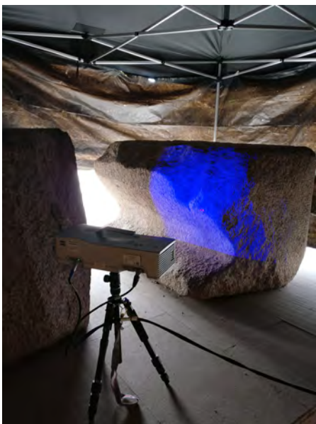
3D scanner ZEISS COMET in action in Tell Basta.
