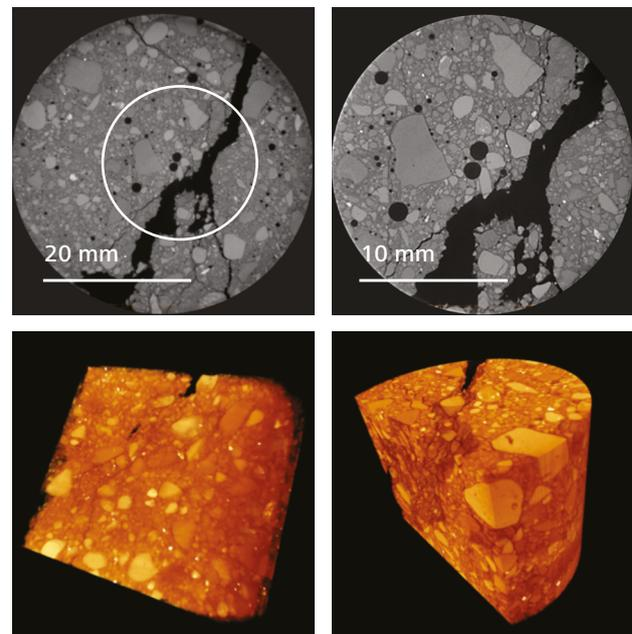
**Figure 2A** (Top Row) Various images showing 20  $\mu\text{m}$  voxel resolution (40mm FOV) on the left and 10  $\mu\text{m}$  voxel size (20 mm FOV) on the right. Both scans were taken on the same, intact, 50 mm sample. (Bottom Row) 3D view of same images
