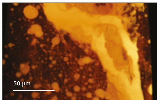
**Figure 1** Inversion of a region of interest in concrete to highlight the cracks and voids.
