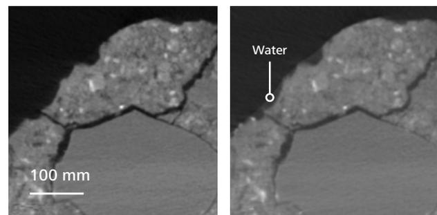
**Figure 3** 4D study under environmental conditions. High contrast enables view of wetting effect.
