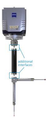
Standard adapter plate with separate extension The standard adapter plate is equipped with a cube to which the extension is screwed on to, as illustrated in the image by the blue frames. However, this additional interface between the cube and the extension reduces the stiffness of the stylus system.
