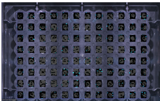
Overview image of a 96-well plate showing the exact position of the obtained transmitted light and fluorescence images.
