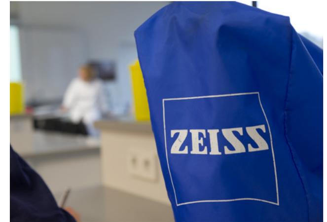
Use a dust cover when microscope is turned off and not in use. Please make sure that the halogen lamp housing is no longer hot before you put the cover on. For long-term storage, microscopes should be kept with a dust cover, if possible in a cabinet. Microscopes should not be kept in styrofoam boxes for a long time.
