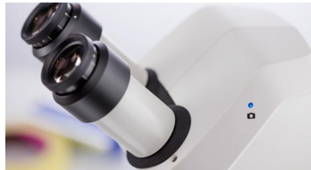
The openings of the binocular viewing tubes must always be closed. Unless the eyepieces are in, use dust stoppers.
