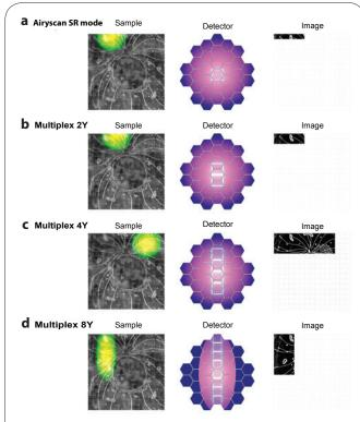
Figure 2 | Depictions of the image-acquisition schemes available on the new Airyscan 2. a, Standard Airyscan SR (super-resolution) imaging. b, Available on LSM 900, the Multiplex 2Y mode acquires two image pixels in parallel. c, Available on both LSM 900 and LSM 980, the Multiplex 4Y mode acquires four image pixels in parallel. d, Available on LSM 980, the Multiplex 8Y mode acquires eight image pixels in parallel.
