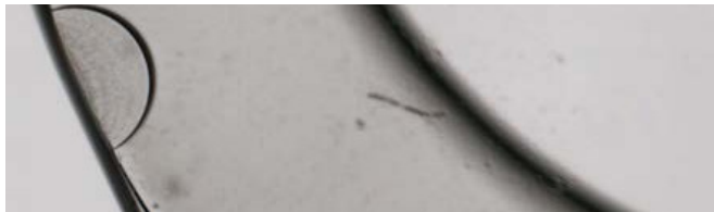
An intraocular lens (IOL), imaged with transmitted light.
