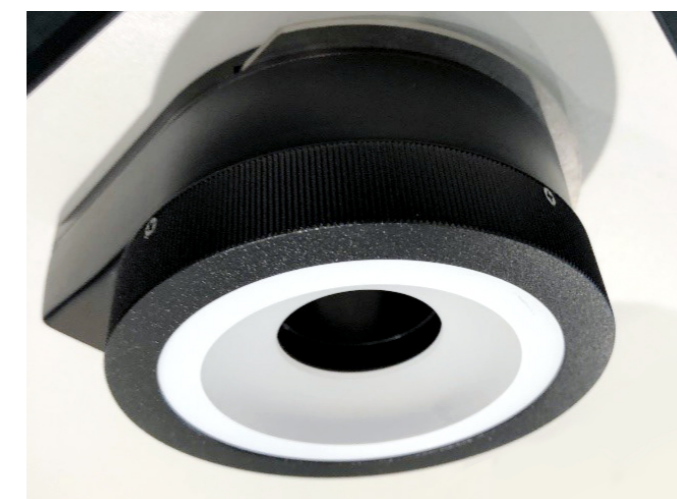
Diffuse light option on ZEISS O-DETECT
