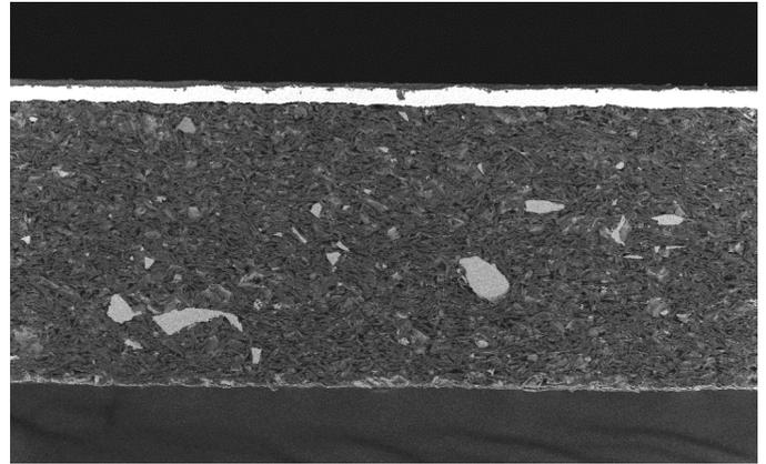
BATTERY ANODE CROSS-SECTION
