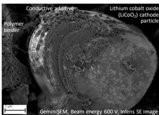
BATTERY CATHODE PARTICLES
