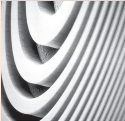
Figure 5. SEM image of Fresnel zone plate
