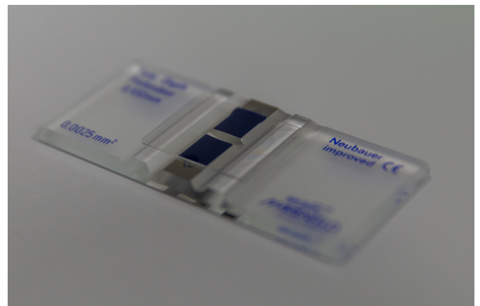
Figure 11 Neubauer improved hemocytometer
