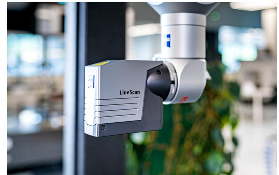
The use of optical sensors like ZEISS DotScan – a confocal white-light sensor – or laser triangulation sensors as ZEISS LineScan allow to measure battery tray features with high speed and high accuracy.
