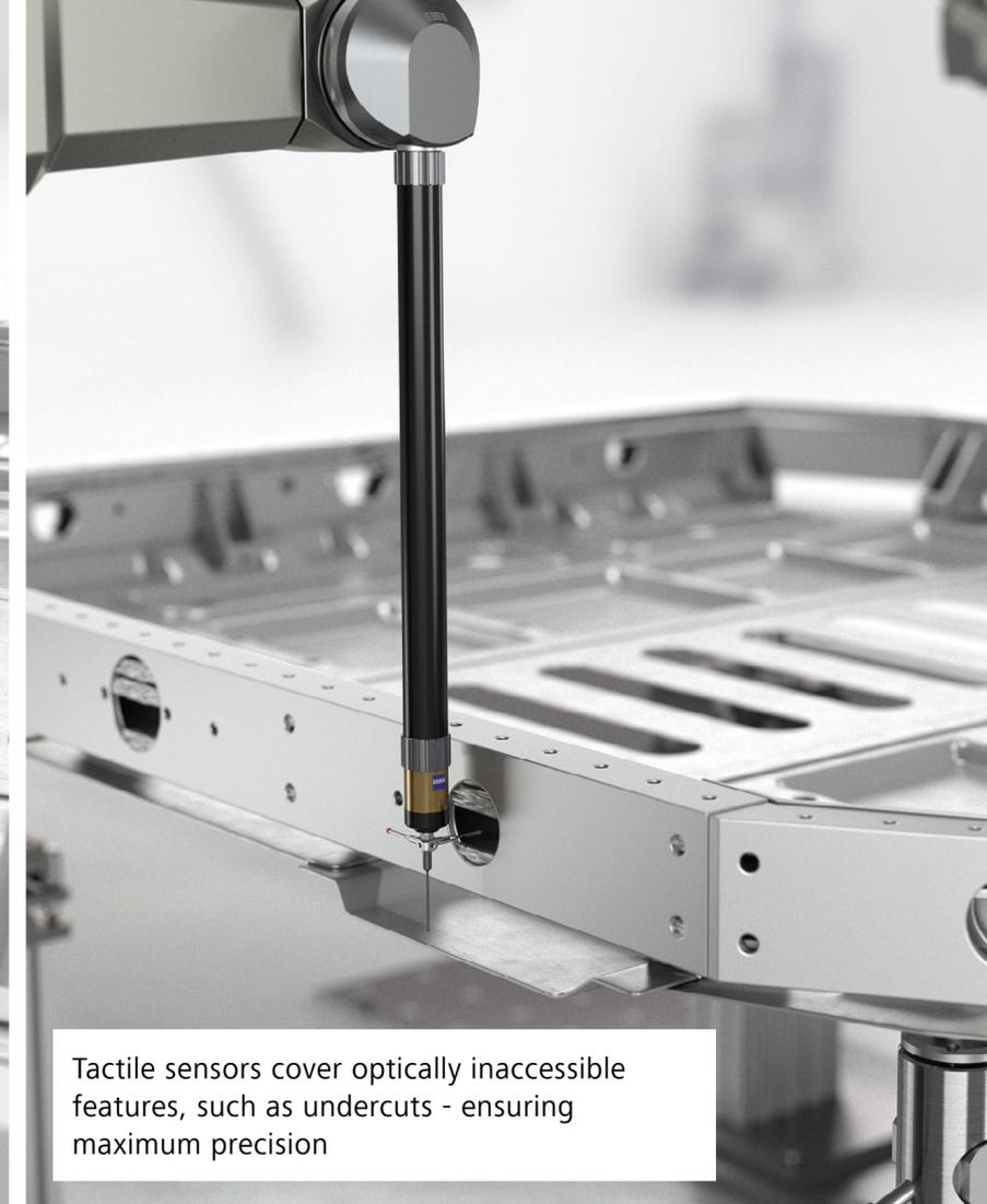
Tactile sensors cover optically inaccessible features, such as undercuts - ensuring maximum precision
