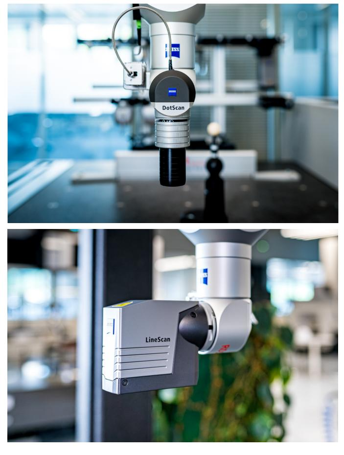
The use of optical sensors like ZEISS DotScan – a confocal white-light sensor – or laser triangulation sensors as ZEISS LineScan allow to measure battery tray features with high speed and high accuracy.
