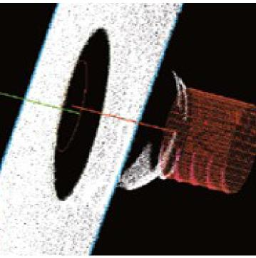
Measurability of complex features: Nut behind sheet Metal
