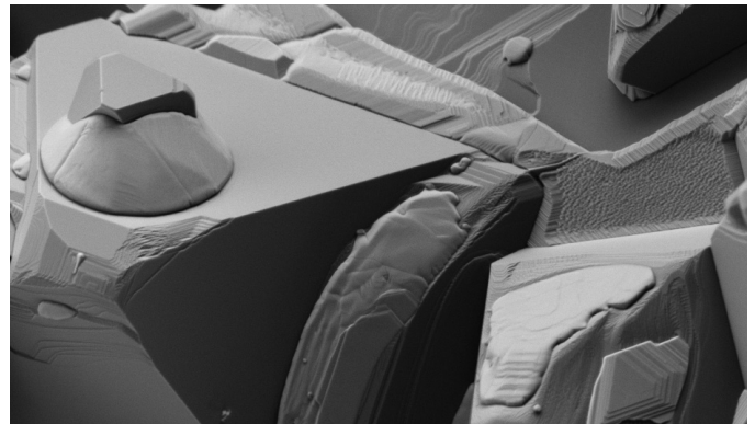
Compositional contrast generated by various materials, taken with the EsB Detector.
