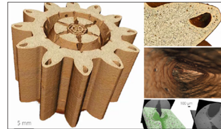
3D scan of Al component produced by additive manufacturing and, inset, internal porosity imaged via X-ray microscopy
