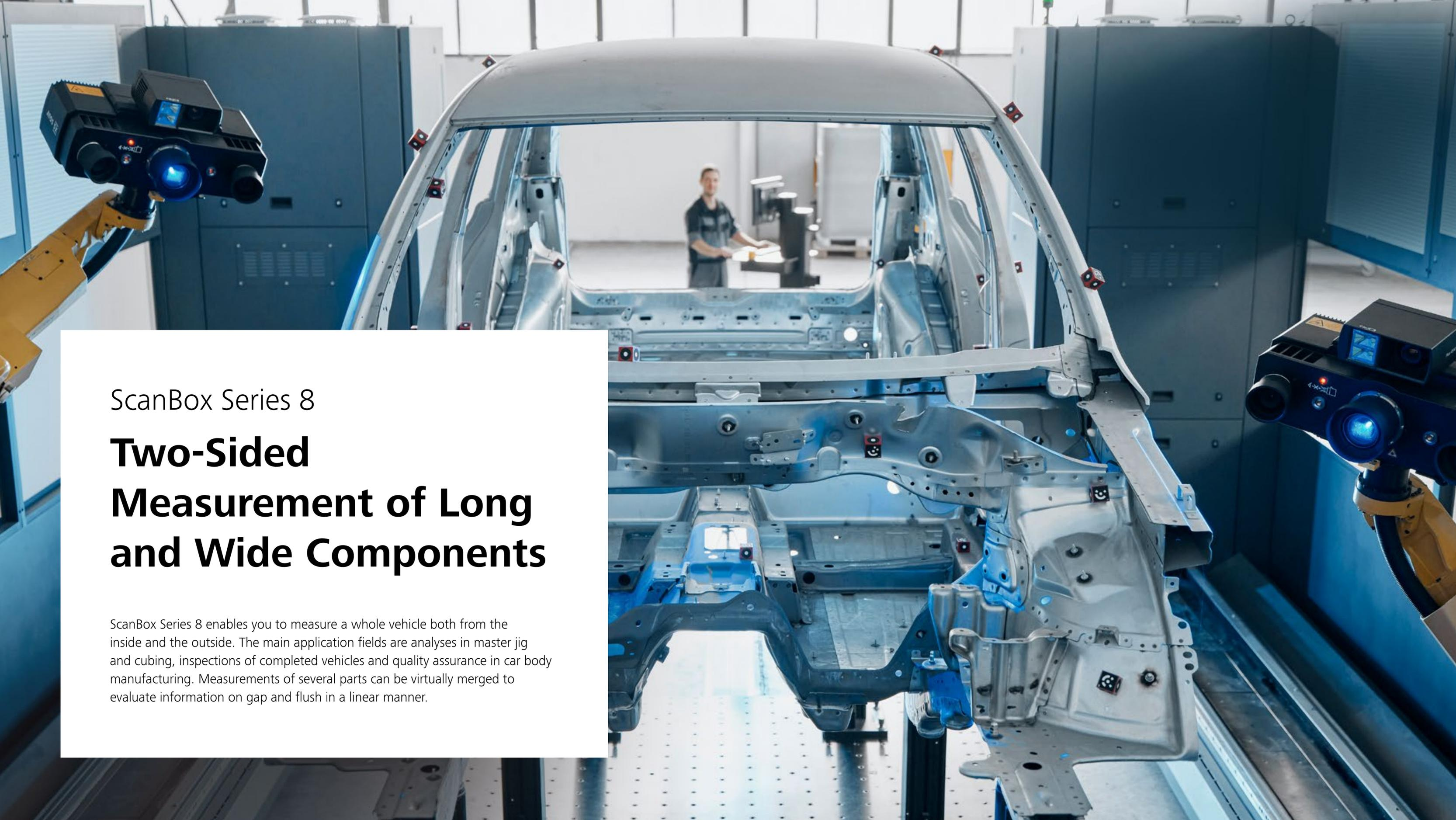
A car body is positioned on a production line in a factory. Two robotic arms, one on the left and one on the right, are equipped with blue laser sensors (ScanBox Series 8) that are scanning the car's exterior and interior. The car body is light blue and has several red markers attached to it. In the background, a worker is visible, and the factory environment is clean and well-lit.
